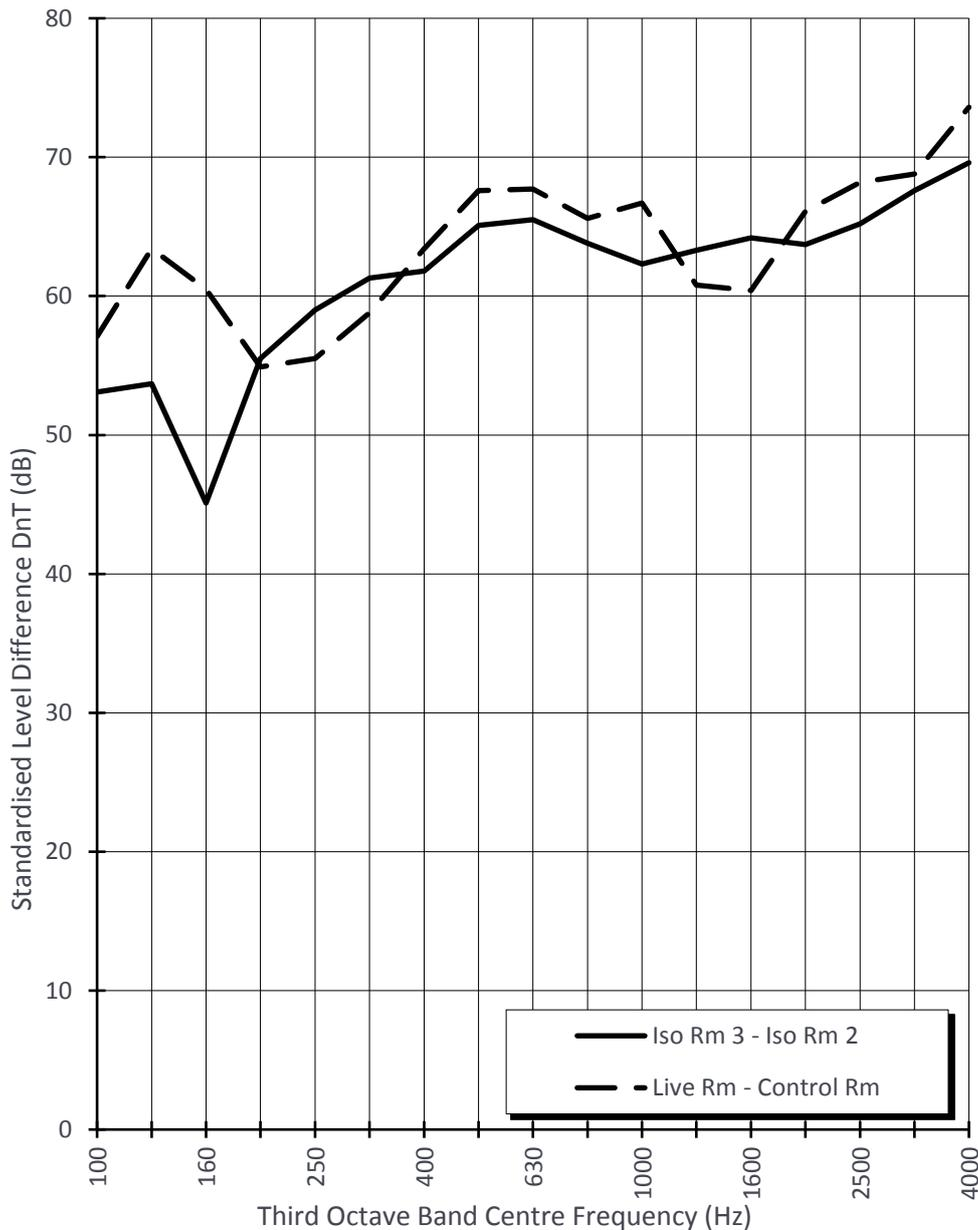
Figure 5: Transmission Loss tested on completion
